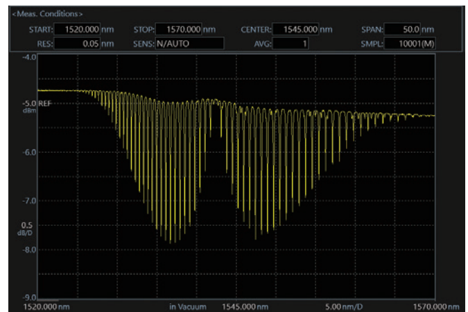
Hydrogen Cyanide \text{H}_3\text{C}_{14}\text{N} absorption spectrum measurement with AQ6375E
